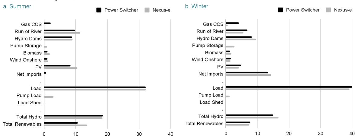
**Figure 8:** Comparison of seasonal electricity generation in 2040 in the Baseline Scenario in **a.** summer and **b.** Winter. The value for load presented here does not include efficiency losses for pumps and batteries.
